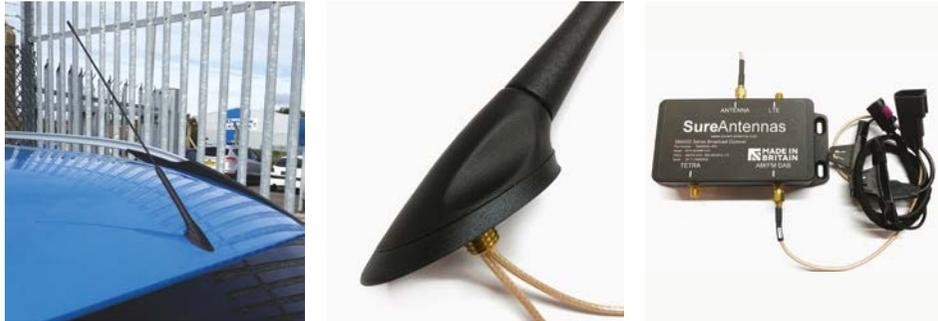
Sure Antennas are able to modify the genuine vehicle antenna from any car manufacturer to your specification providing a truly covert solution. The antenna on this page is from a 2017 Ford Transit Connect van that came from a customer's multi-functional requirement.
