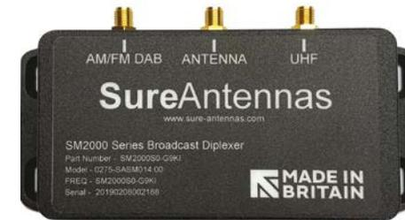
The SM2000 range of Diplexers are designed to provide an improvement of VSWR between a multiple transmitters and one aerial. In order to maintain this enhanced performance it is necessary to minimize insertion losses through the system. The SM2000 is designed with a very low insertion loss factor of less than -0.3 dB at VHF, and Port to Port Isolation of better than -40dB. This, together with its capability to improve
