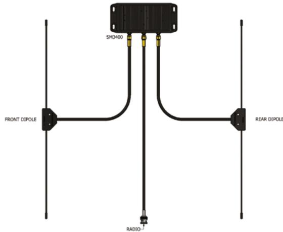
Sure Antennas pair of bumper antennas is an ideal solution for vehicles where a roof mounted antenna is not an option, maybe due to a covert operation or a motorcycle installation. Each front and rear Dipole antenna is produced to your required frequency and individually tested to insure the best possible performance is achieved. Using ultra low loss cabling in the construction of the kit, and a combiner unit improves reception overall and gives an edge to just
