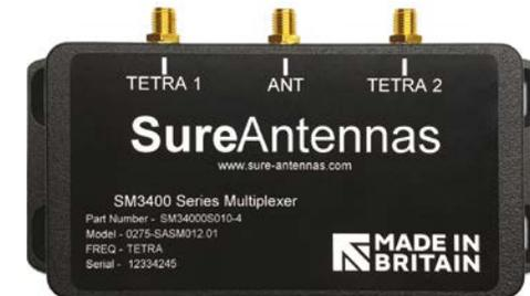
The SM3400 divider / combiner unit was specifically designed to enable two transmitters to transmit simultaneously, without the use of switching circuitry.
