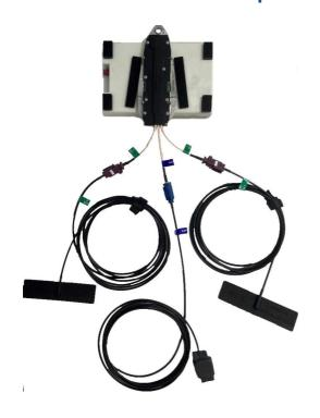
Our OEM Antenna Repositioning Kit is designed for the latest generation of BMW vehicles. This kit replaces the factory-fitted sharkfin antenna with a critical communications antenna, optimising roof space for additional equipment such as antennas or solar panels. It allows the OEM sharkfin antenna to be repositioned while retaining the existing wiring and replacing the original antennas with internal window mounts.
