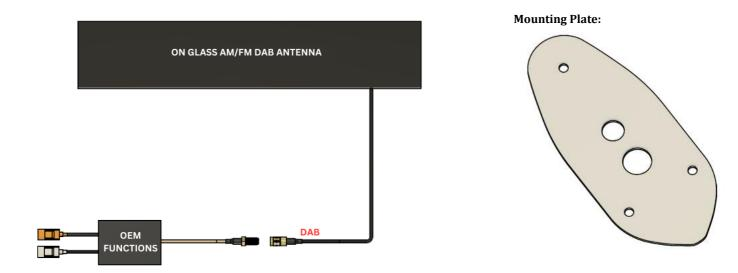
Introducing the **Opel Corsa 'Mallard'/'Sandcastle' Fitting Kit (SK010019)**, designed for versatile installation options tailored to your needs. This **On-Glass AM/FM DAB antenna** can be fitted directly to the glass of a marked vehicle, ensuring **optimal reception**. For a more **discreet installation on unmarked vehicles**, the antenna can be adhered to the inside of the headlining or positioned on the plastic roof spoiler.
